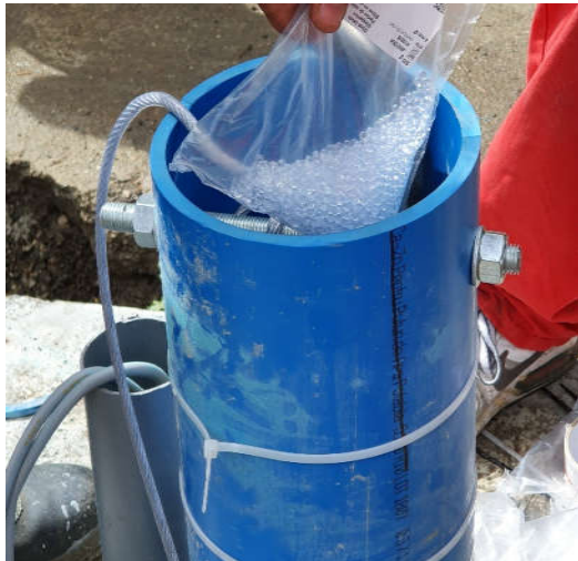
Figure 6. Pouring a bed of glas beads into the protective tube T_{PVC}
