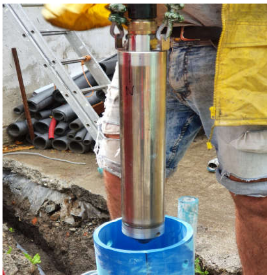
Figure 7. Launch the 3D vibration transducer into the protection tube
