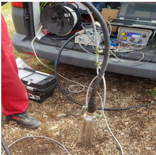
Figure 4. Checking / calibrating the 3D vibration detector - coupling with digitizer K2
